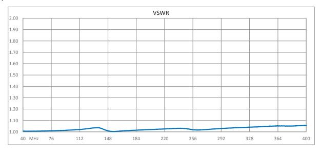
Click the following link (or enter part number in "SEARCH" on website) to obtain additional part information including price, inventory and certifications: Type N F/M Coaxial RF Surge Protector, 40MHz - 400MHz, DC Pass, 100W, IP67, 2.5mJ, 20kA, Hybrid, Bracket Down, Hole Mount BGXZ-60NFNM-ALT
